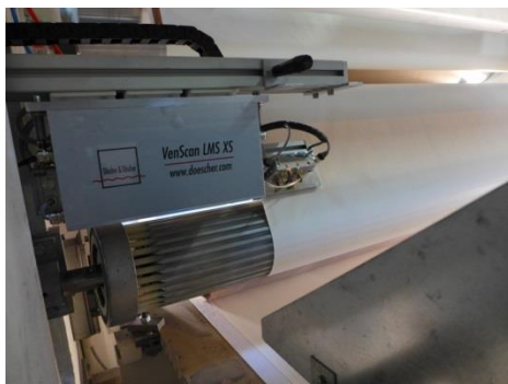
Abb. 18: VenScan LMS XS Sensor
